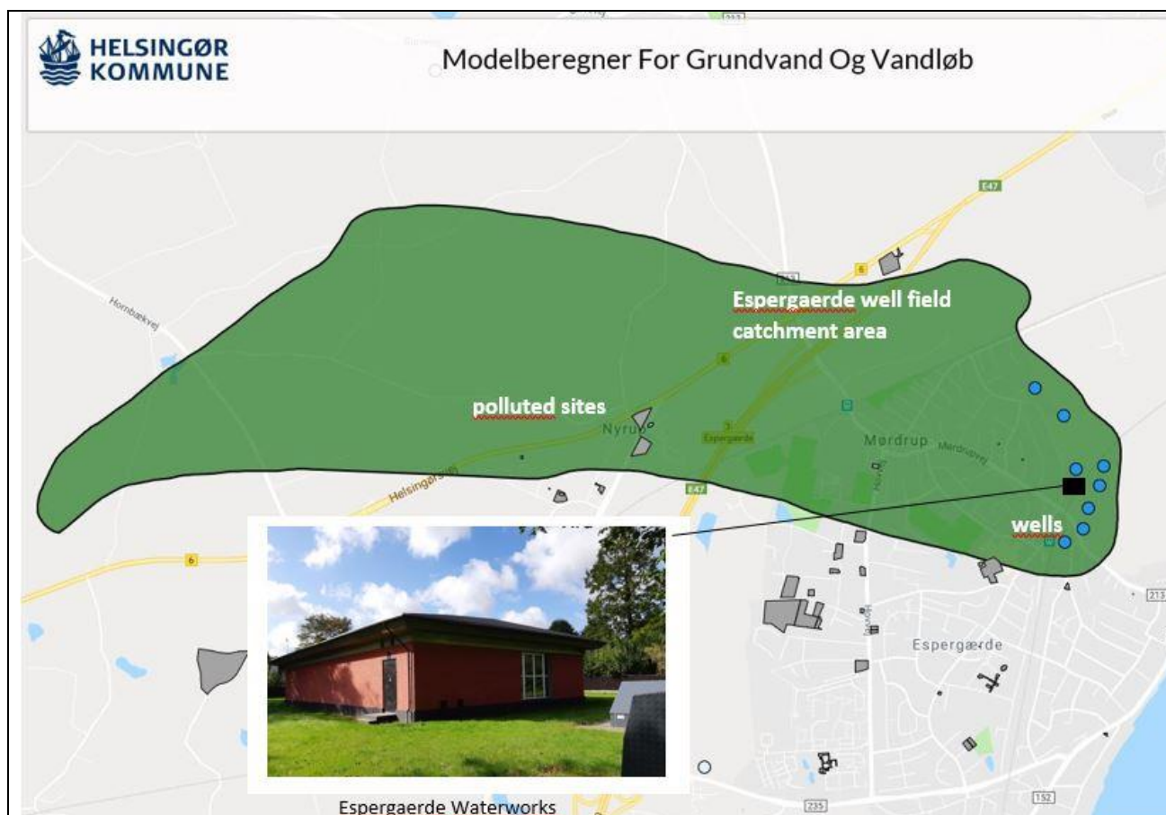
Figure 4.1: Graphical output of the Elsinore decision support tool covering the catchment area to the well field (blue dots) of Espergærde water works (1.200.000 m 3 /year).
